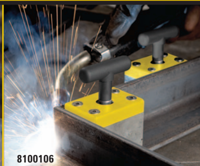
Fabricate angles quickly; pull corners together with hold on multiple sides.
