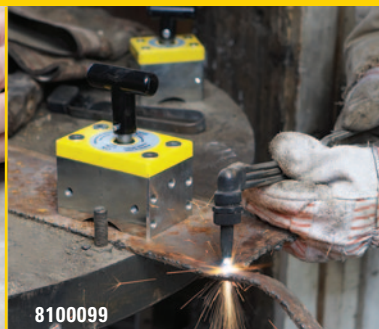
Secure steel for fabricating or cutting.
