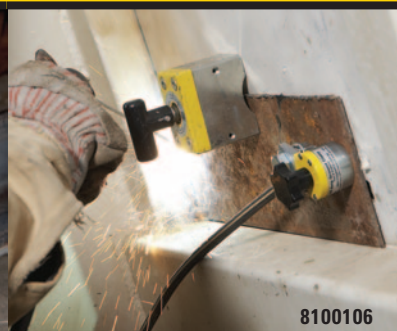
Helping hand – a temporary support to hold a part or tool on a vertical wall.
